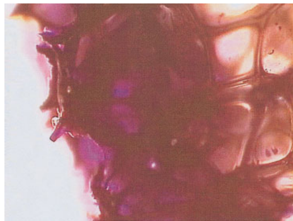
Figure 2. The ELSM photograph of the cross section of the cell-immobilized polyurethane foam (25 × 4 folds).
